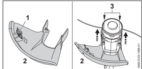
The line limiting blade (1) is already installed in the deflector (2) and must not be removed.
